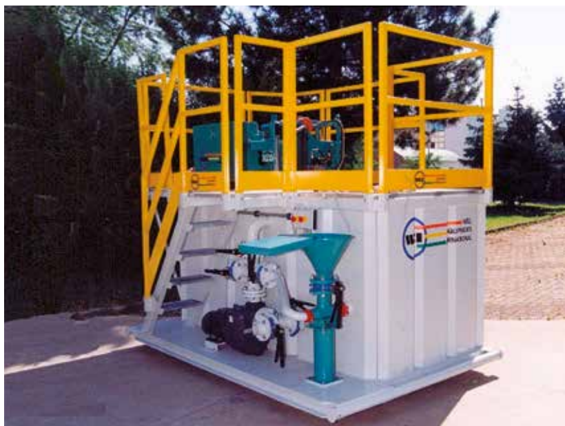
2' x 3 1/2' double screen shale shaker complete of 6m 3 mud treatment group.
